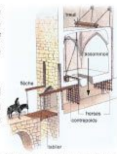
Diagram of the mechanism of a drawbridge counterbalanced
